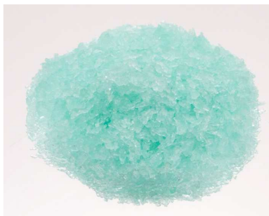
Figure 2. Melanterite obtained from the biohydrometallurgical/UV processing of the coal tailing.
